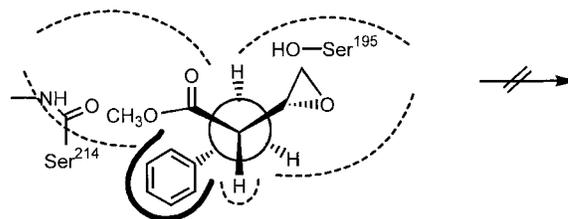
**FIGURE 3** (2*S*,3*S*)-2-Benzyl-3,4-epoxybutanoic acid methyl ester anchors in the active site of  $\alpha$ -chymotrypsin with the oxirane moiety being positioned in the catalytic site, but the C<sub>3</sub>—O bond is not aligned favorably for the S<sub>N</sub>2 type ring cleavage reaction. No nucleophilic attack of the Ser-195 hydroxyl on the oxirane ring ensues.
