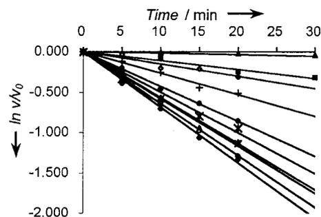
**Figure 2.** Plot of  $-\ln(v/v_0)$  vs incubation time, showing time-dependent loss of CPA activity by ( $\alpha,4R$ )-**1** ( $\blacklozenge$ ,  $[I]_0 = 30$  mM;  $\circ$ ,  $[I]_0 = 28$  mM;  $\triangle$ ,  $[I]_0 = 26$  mM;  $\times$ ,  $[I]_0 = 24$  mM;  $*$ ,  $[I]_0 = 22$  mM;  $\bullet$ ,  $[I]_0 = 20$  mM;  $+$ ,  $[I]_0 = 18$  mM;  $\diamond$ ,  $[I]_0 = 16$  mM;  $\blacksquare$ ,  $[I]_0 = 14$  mM;  $\blacktriangle$ ,  $[I]_0 = 0$ ).
